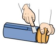
• Carefully file away the cable carrying strip until flush with the riser.
